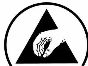
The ESD Protective Symbol identifies products designed to provide ESD control protection.
