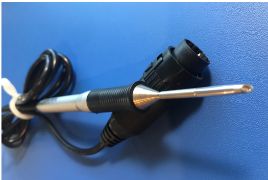
Figure 4. WXMP iron with GW tip
