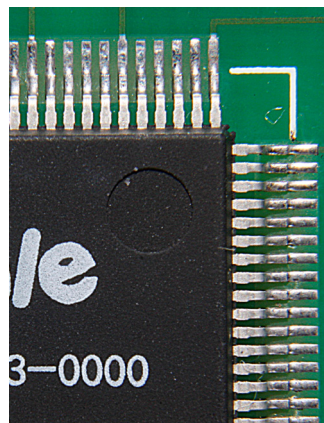
Figure 1: Top view of the corner of a QFP
