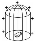
To complete the enclosure, make sure to place lids on boxes or containers, and close shielding bags. Packaging with holes, tears, or gaps should not be used as the contents may be able to extend outside the enclosure and lose
